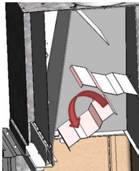
Figure No.28 - Removing the middle deflector on the Itaca
