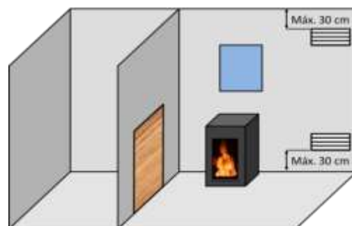
Figure No. 4 - Guideline indications for ventilation grilles
