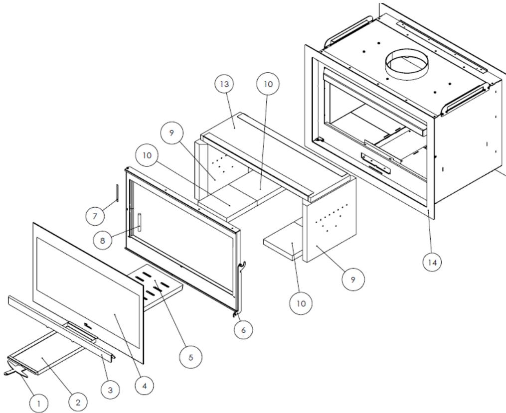
Figura n°23 - Pezzi principali Nickel 700/800/1000
