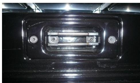
Figure No.19 - Accesses via which to clean the flue socket.
