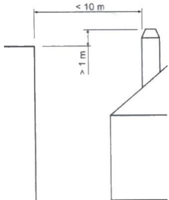
*Figure No.3 - Distances between the chimney crown and objects within a 10m radius*
