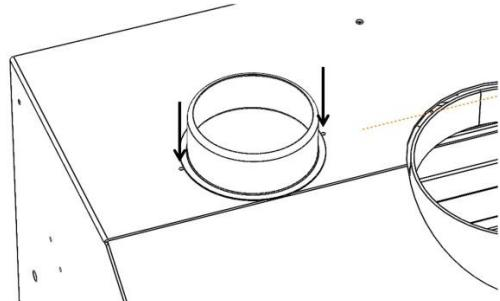
Figure No.9 - Screw the nozzle.
