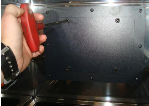
Figure No.17 - Access to the screws to remove the hatch cover
