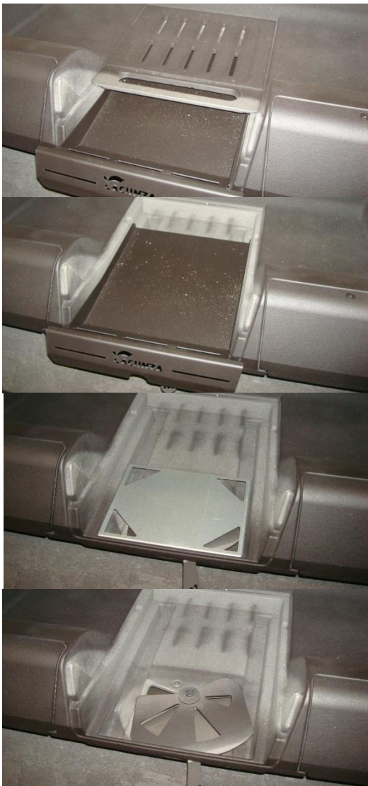
Figure No.25 - Disassembly of pieces for cleaning access
