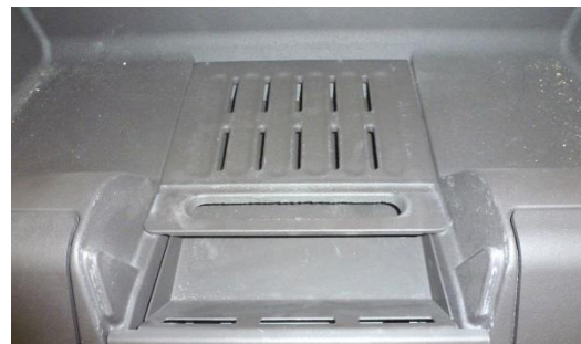
Figure No.24 - Removed separator
