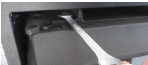
Figure No.10 - Loosening the door support with a 10 mm wrench
