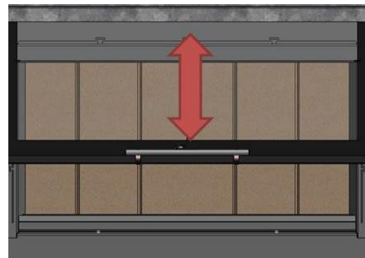
Figure No.36 - Opening using guillotine system
