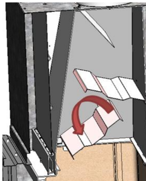
Figure No.32 - Removing the middle deflector on the Itaca
