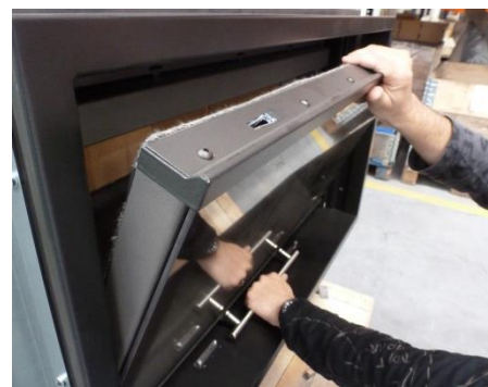
Figure No.41 - Hold the door firmly with both hands as you lower it
