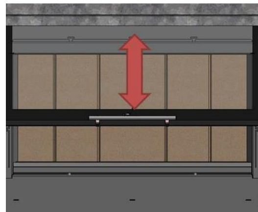
Figure No.32 - Opening using guillotine system
