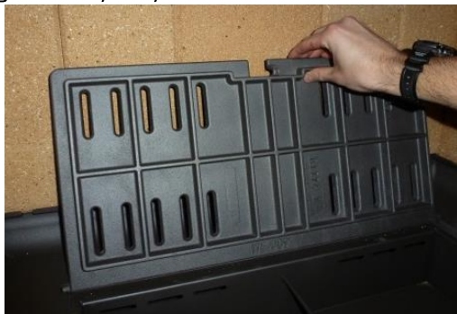
Figure No.24 - Rest grille against the back of the firebox
