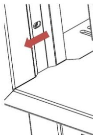
Figure No.11 - Unscrew the 6 screws that secure the exterior frame
