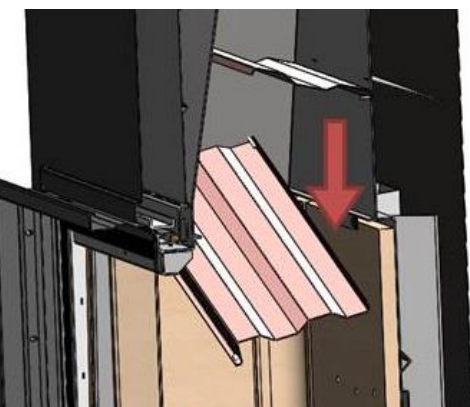
Figure No.25 - Dismantling the lower Inca deflector
