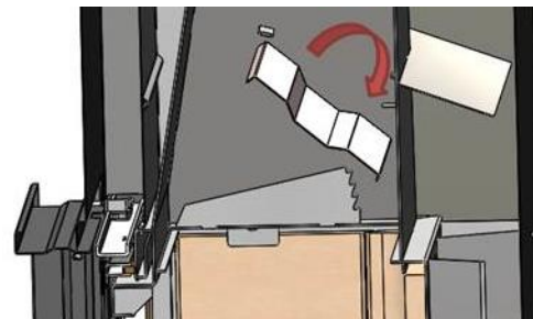
Figure No.26 - Removing the middle deflector on the Inca
