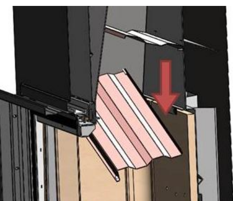
Figure No.25 - Dismantling the lower Inca deflector
