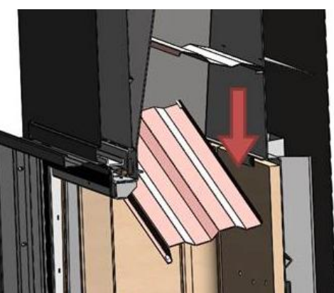
Figure No.25 - Dismantling the lower Inca deflector
