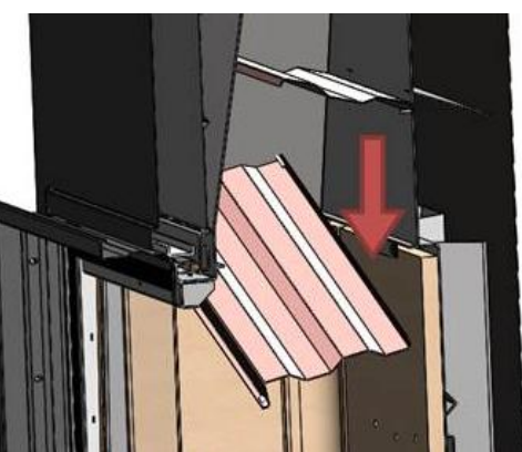
Figure No.25 - Dismantling the lower Inca deflector
