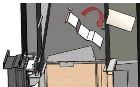
Figure No.21 - Removing the middle deflector on the Inca
