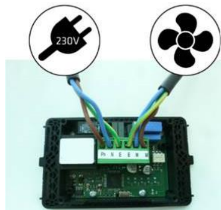
Figure No.26 - Connections to be carried out in the potentiometer
