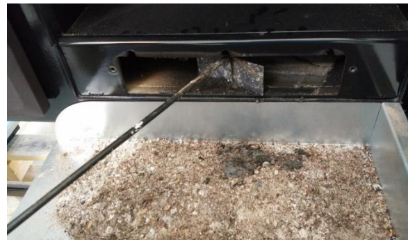
Figure No.18 - Accesses via which to clean the flue socket.
