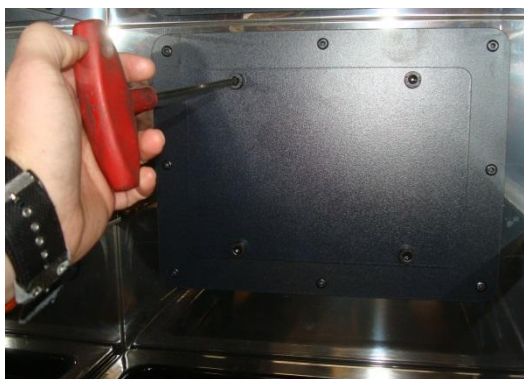
Figure No.21 - Access to the screws to remove the hatch cover
