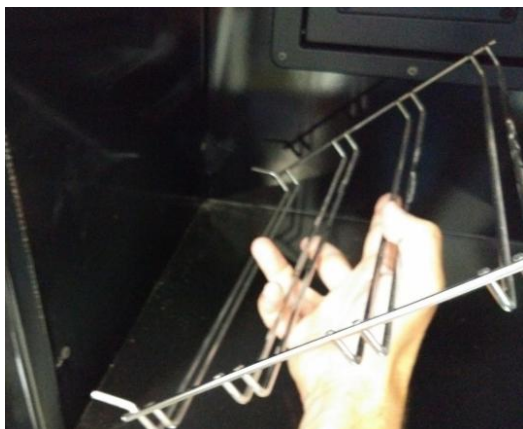
Figure No.23 - Removal of the brackets and self-cleaning sides
