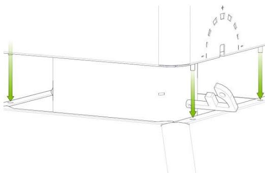
*Figure No.5 - Lower tube cover positioning*
