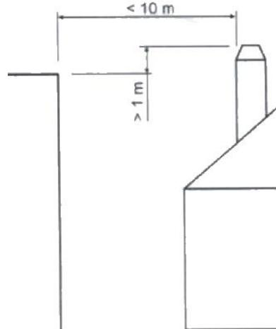
*Figure No.8 - Distances between the chimney crown and objects within a 10m radius*
