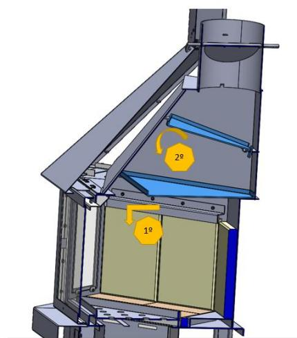
Figure No.1 - Dismantle the steel defectors
