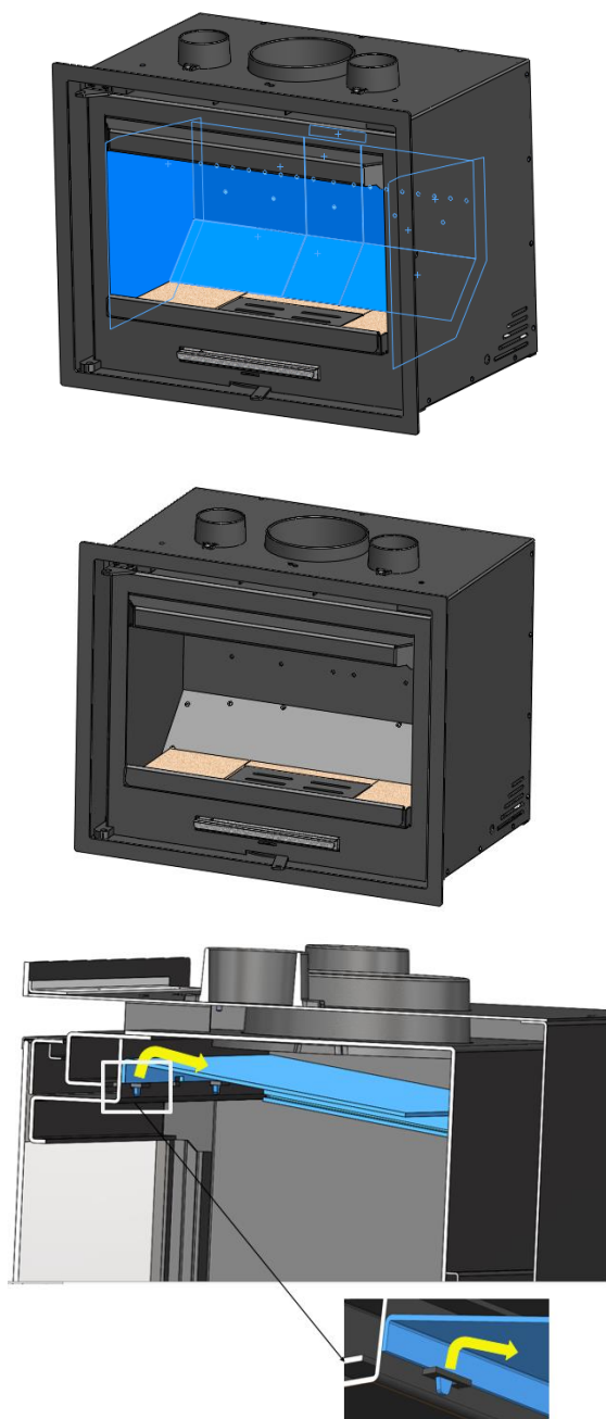
Figure No.9 - Dismantling the ADOUR steel deflector
