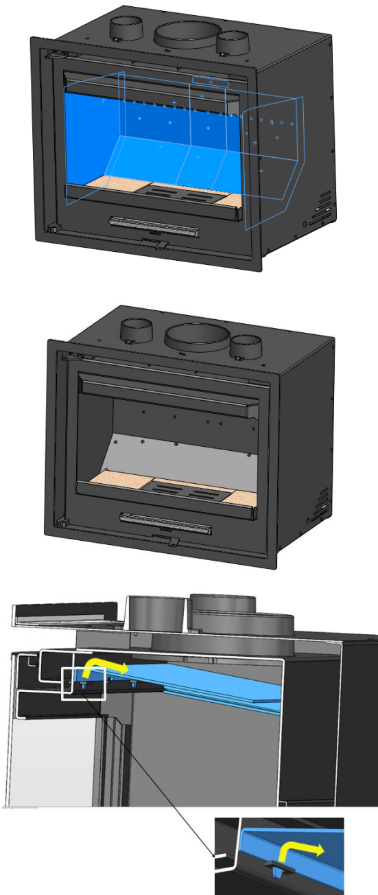
Figure No.9 - Dismantling the ADOUR steel deflector
